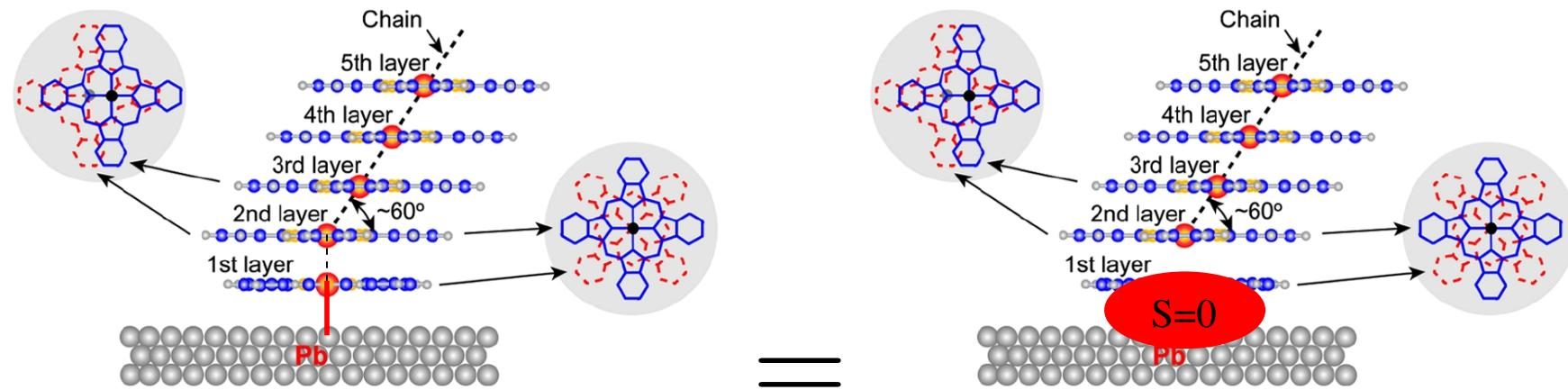
Stack of deposited Cobalt phthalocyanine (CoPc) molecules;
