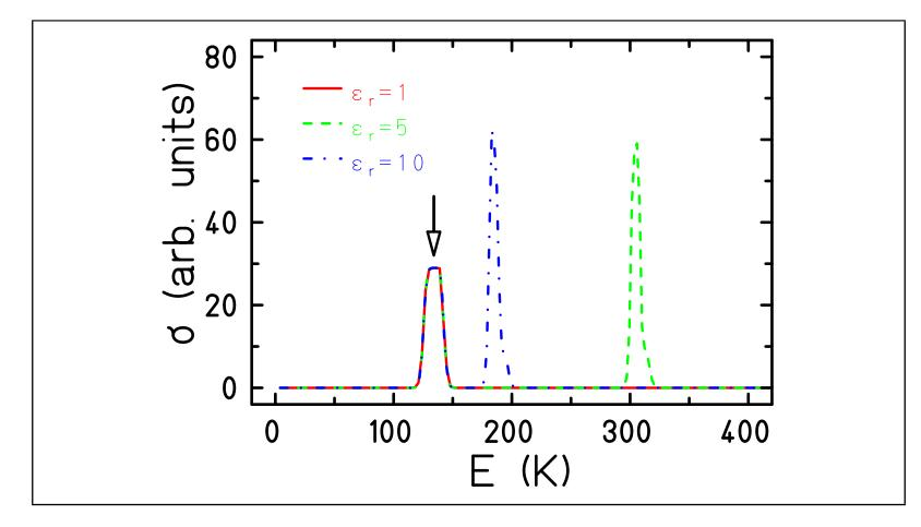
Rough sketch of the lowest transitions observable with inelastic neutron scattering. The arrow marks the singlet-triplet transition at about 135 K.
